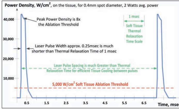
Figure 8. SuperPulse explained: High power, short laser pulses maximize soft tissue removal rate and keep adjacent tissue cool.
