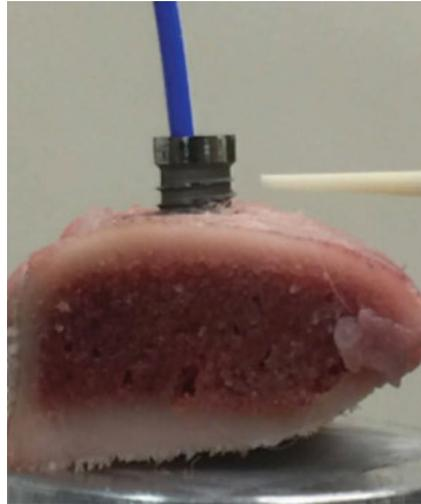
Figure 9: NanoTite™ implant embedded in a block of pork rib bone and irradiated by CO<sub>2</sub> laser
