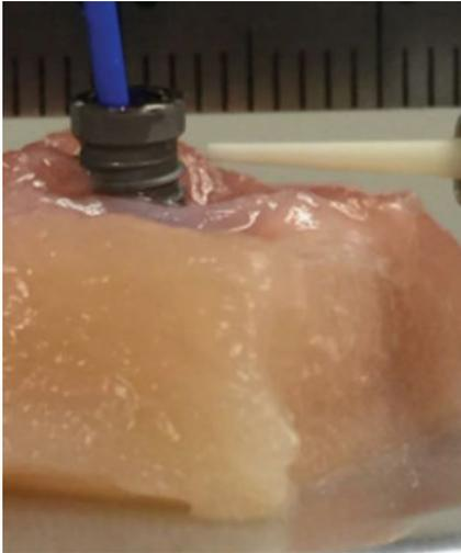
Figure 8: NanoTite™ implant embedded in a block of poultry soft tissue and irradiated by CO<sub>2</sub> laser
