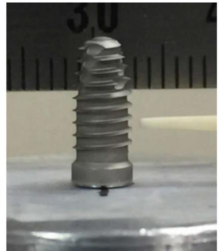
Figure 1: Implant centered on the rotating platform. 10,600 nm CO<sub>2</sub> laser beam from the Perio Tip (on the right) is directed at the implant surface
