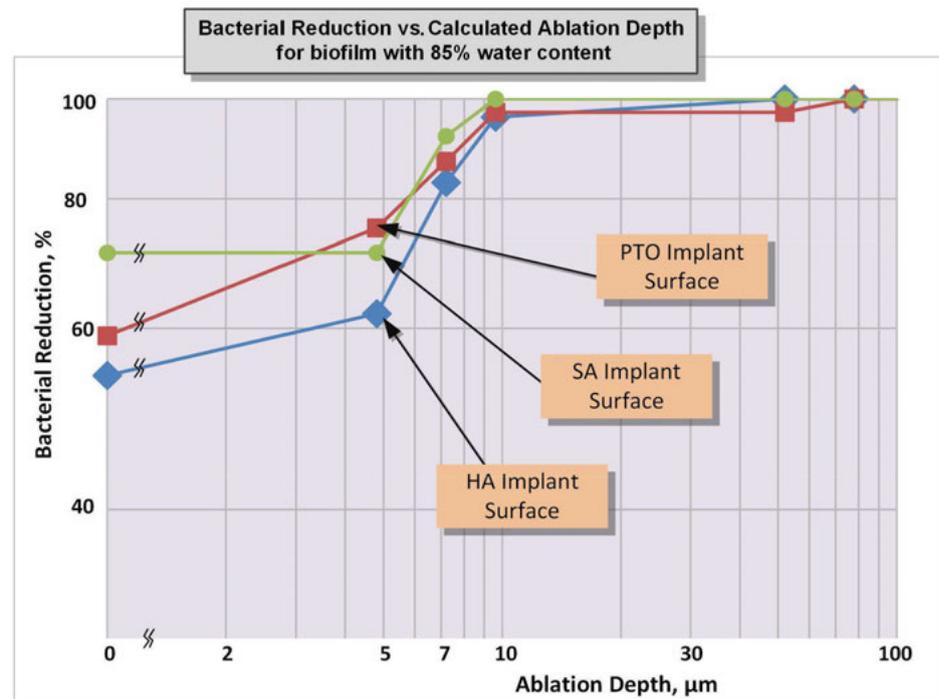
Figure 5: Bacterial reduction vs. calculated ablation depth for 10 μm thick biofilm with an assumed 85% water content
