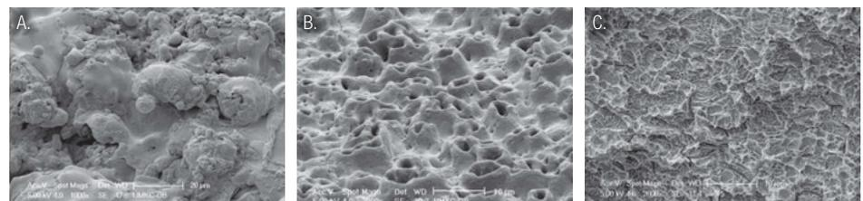
Figure 1: Untreated implant surfaces with no biofilm: (1A) HA plasma-spray coated. (1B) Untreated PTO. (1C) Untreated SA. Original magnification of x1,000; bar = 20 μm (1A); and x2,000; bar = 10 μm (1B, 1C)
