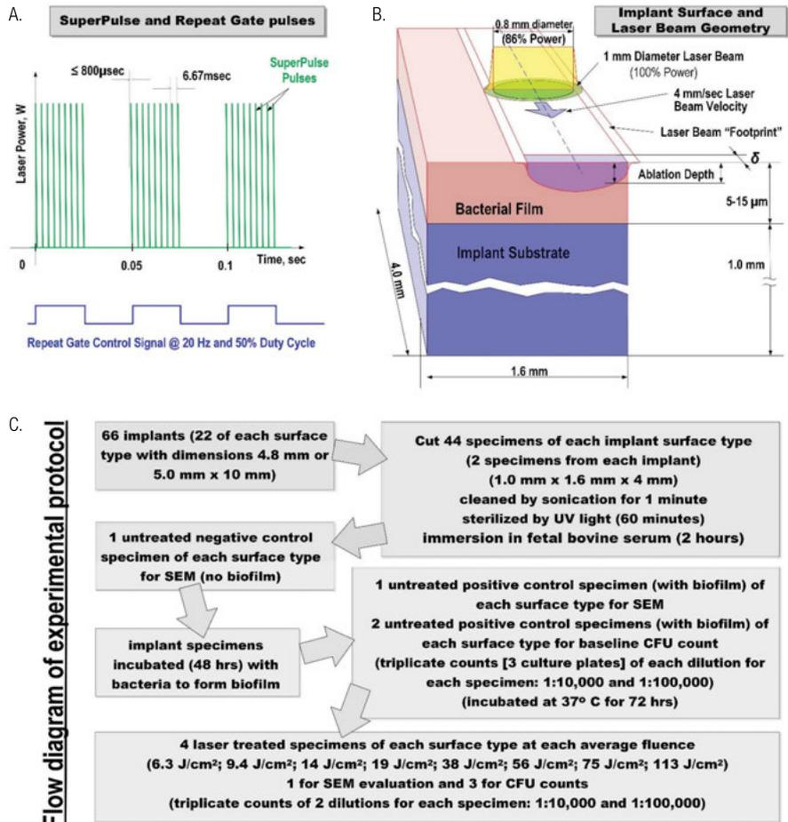
Figure 2: Drawings depicting (2A) repeat gating of SuperPulse modes with longer pulses (≥ 10 msec) at lower frequencies (≤ 30 Hz); (2B) movement of the laser beam over the biofilm adhering to the implant surface; and (2C) schematic of experimental protocol
