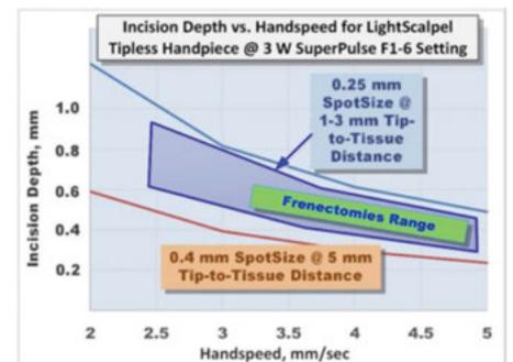
Figure 7: Ablation depth in water-rich soft tissue with LightScapel's tipless dental handpiece at 3 watts in the SuperPulse (150 Hz, 26.7 mJ) Repeat F1-6 (20 Hz, 30 msec) mode
