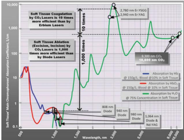
Figure 4: Optical absorption coefficient spectra at different histologically relevant concentrations of water, hemoglobin (Hb), oxyhemoglobin (HbO<sub>2</sub>), and melanin
