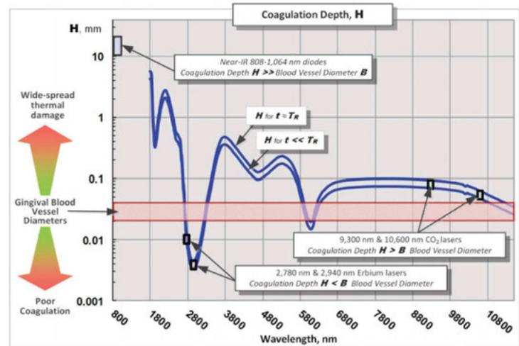
Figure 5: Coagulation depth spectrum for pulsed laser ablation from Vitruk<sup>29</sup>;  $T_r$  is Thermal Relaxation Time<sup>29,30</sup>
