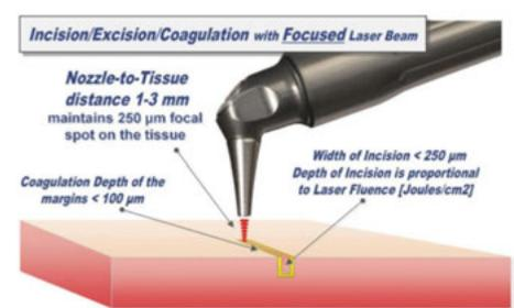
Figure 6: Laser-tissue incision with focused (0.25 mm spot size) laser beam. Defocused beam (approximately 0.8 mm spot size) with reduced fluence coagulates the tissue. The handpiece is pen-sized, autoclavable, and uses no disposables
