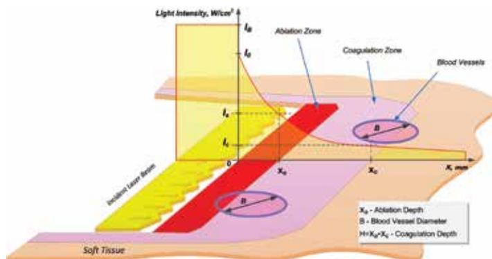
Figure 2: Simplified graphical representation of laser beam intensity attenuated inside the soft tissue
