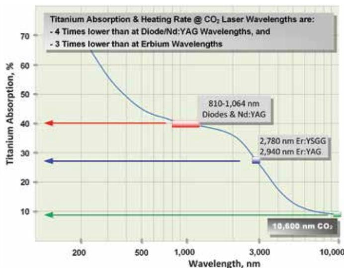
Figure 3: Titanium surface optical absorption spectrum derived from Wolfe and Zissis<sup>17</sup>
